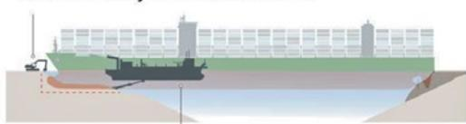
Dredgers dug sand and mud from under the bow and stern up to a depth of 18 m
